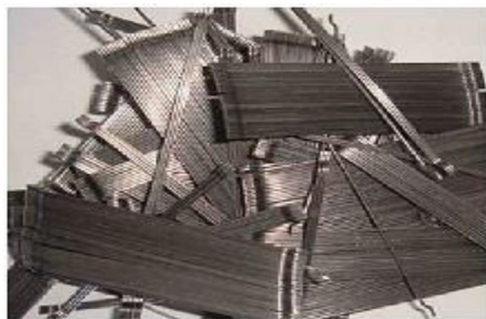
Fig. 1. Photos of Glued DRAMIX Steel Fiber and Polypropylene Fiber.
